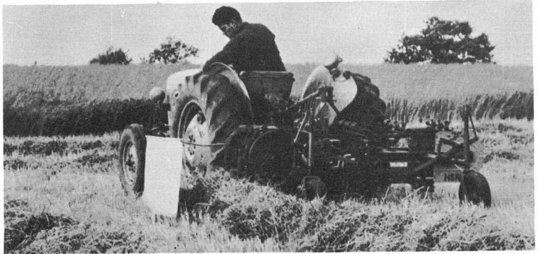
Combined haymaker from the JF Machine Factory, shown here turning swaths.
